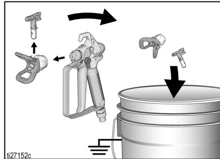
4. Wipe paint off outside of gun using a soft cloth moistened with water or flushing fluid.
