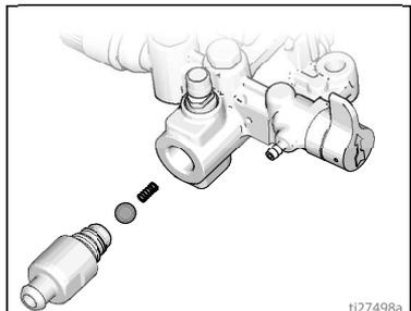
3. Clean any debris and dried paint from the cavity and replace the ball and spring. Tighten inlet valve to pump using integrated tool on the frame.
