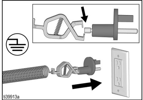
**Fluid hoses:** Use only electrically conductive hoses with a maximum of 300 ft. (91 m) combined hose length to ensure grounding continuity.
