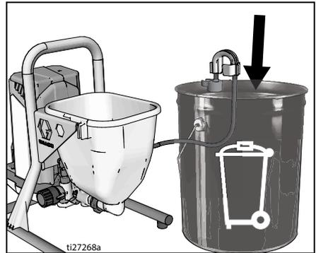
6. Pour flushing fluid into the hopper. Use water for water-based paint and mineral spirits for oil-based paint.
