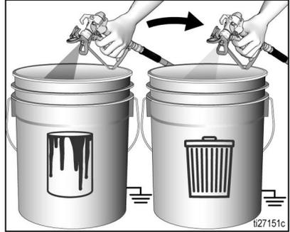
15. Stop triggering gun. Engage the trigger lock.
