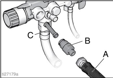
5. Check InstaClean Fluid Filter (C) for debris. If needed, clean filter with water or flushing solvent and a soft brush.
