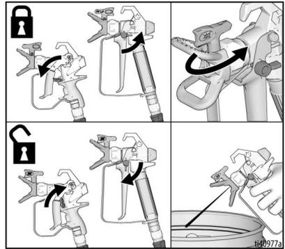
2. Engage trigger lock. Rotate spray tip back to spray position. Disengage trigger lock and continue spraying.
