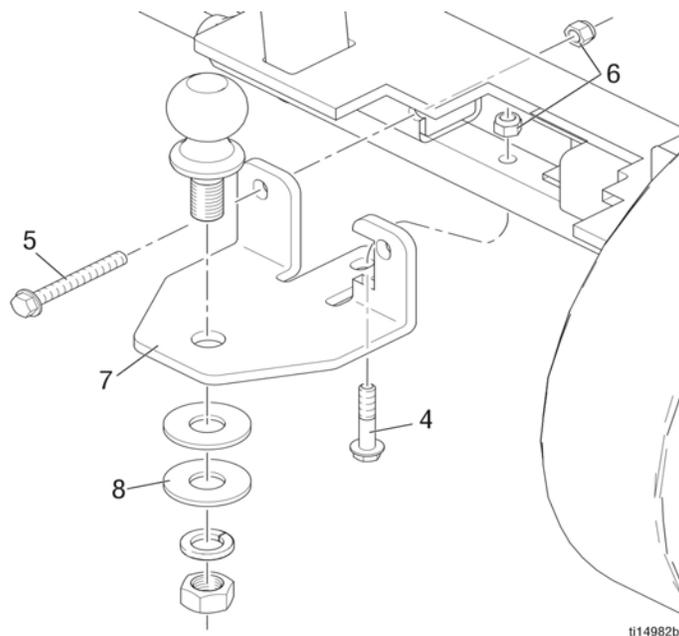
1. Remove ball from standard hitch assembly.
