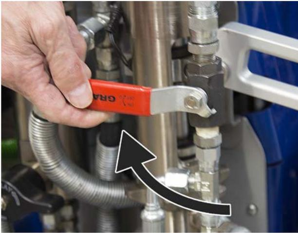
2. Open hydraulic valve on solvent pump.
