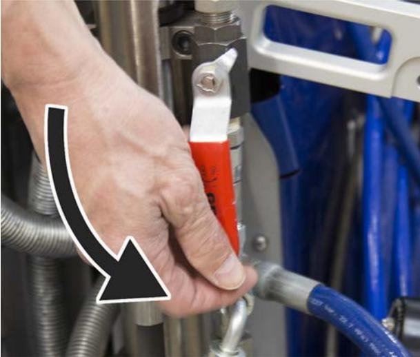
13. Open material supply lever (B) on mix manifold.
