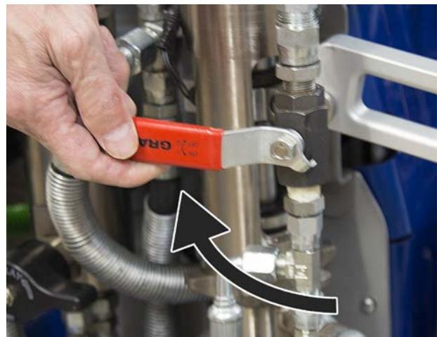
11. Move resin (MMA) Spray/Prime valve (C) to SPRAY position.
