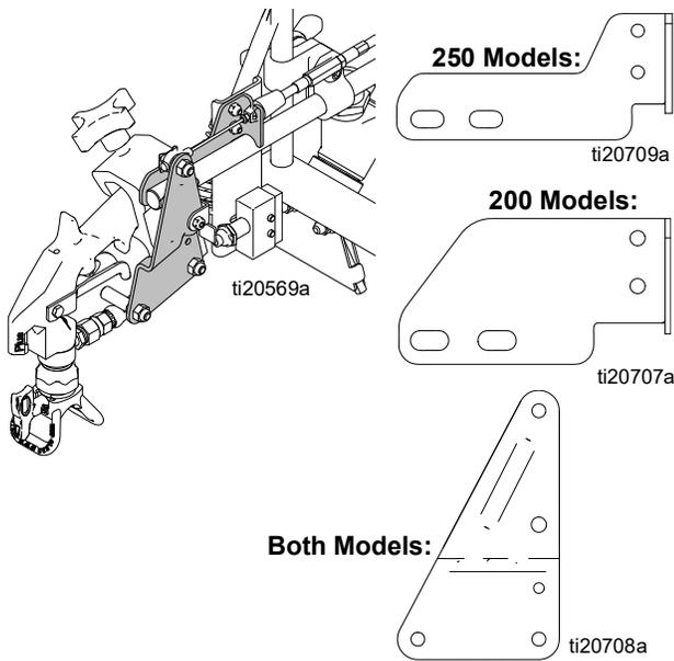
2. See **Parts** diagram to assemble bead gun accessory parts, page 5.
