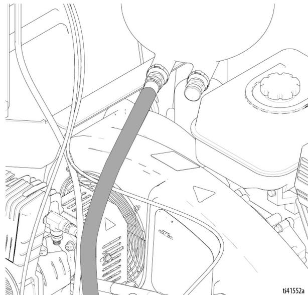
7. Push one end of remaining air line into top hole on air switch and run along bead hose to tank and then route and push into elbow fitting (J) on air tank.
