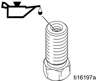
8. Install seat nut, o-ring, and gun needle.
