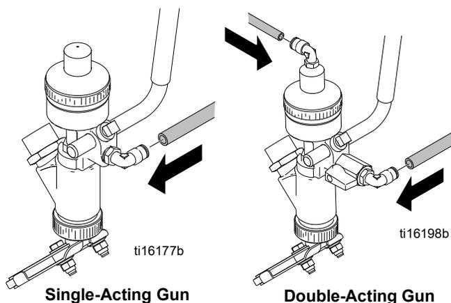
Clean all lines and connections of dirt, burrs, etc. and blow them out with clean air before connecting them to the system. Install an air filter in the air supply line to remove harmful dirt and moisture from the compressed air.
