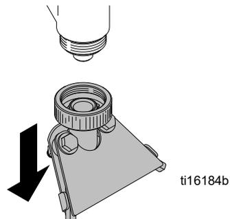
4. Remove valve seat and o-ring from valve housing and remove gun needle.
