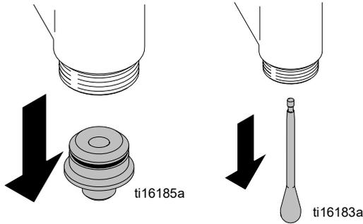
5. Remove seal nut and o-ring.
