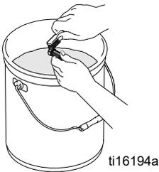
7. Lubricate o-ring with one drop of oil. Install o-ring.
