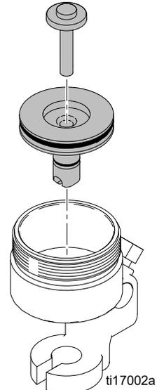
Check the piston o-rings carefully. Lubricate all parts with a light waterproof grease and reassemble the valve using new parts as necessary.
