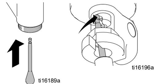
9. Install o-ring on valve seat and insert into valve housing.
