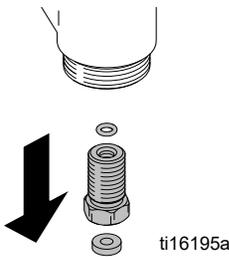
6. Clean all parts. Inspect o-rings for signs of wear, replace as necessary.
