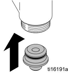
10. Install retaining nut.
