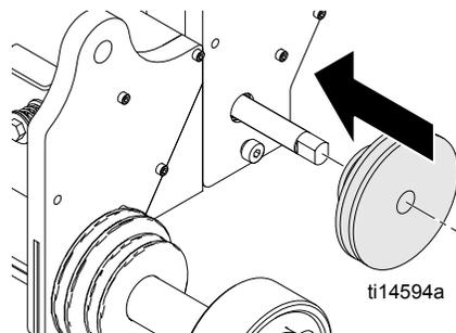
9. Install belts onto pulleys.
