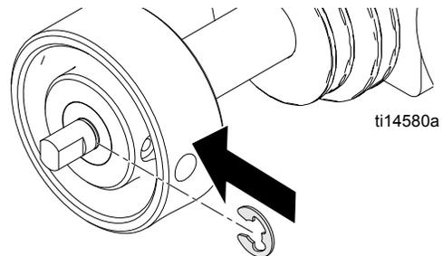
8. Slide pulley onto short axle.
