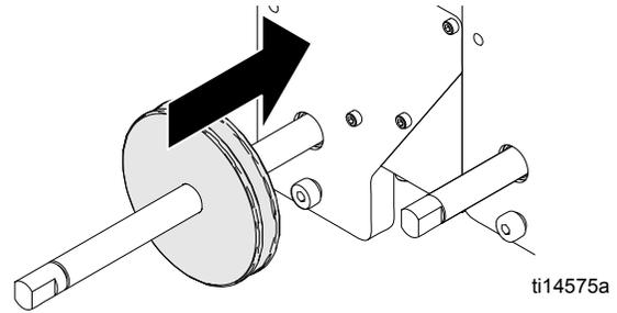
6. Slide bead dispenser engagement wheel pulley onto long axle.
