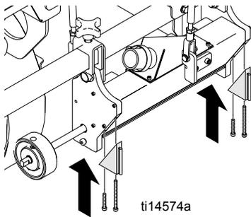
4. Slide double bead box down through slots on angular brackets and lock into place.
