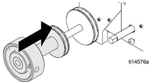
7. Secure pulley and wheel into place with clamp (engagement wheel pulley will still be able to rotate freely).
