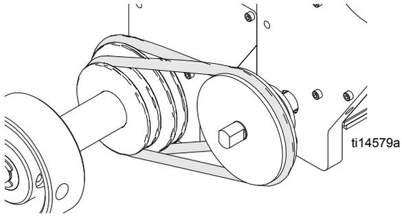
11. Attach pulley guard and tighten two screws.
