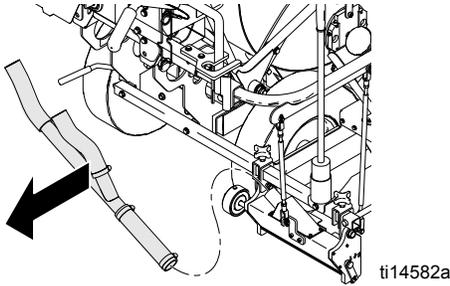
2. Loosen screw and remove bead dispenser engagement wheel.
