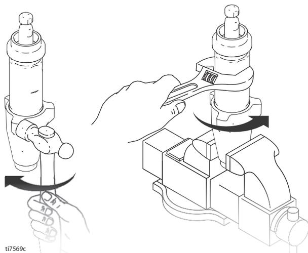
3. Disassemble intake valve. Clean and inspect o-ring (227). **NOTE:** A pick may be required to remove o-ring.
