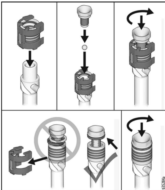
2. Install ball (206) in piston rod. If thread sealant is applied to piston valve threads, make sure that none gets on ball.
