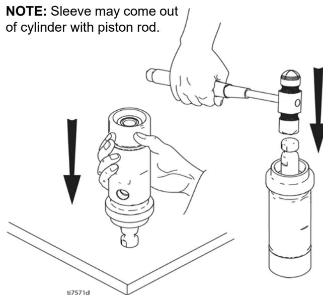
**NOTE:** Sleeve may come out of cylinder with piston rod.
