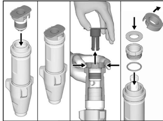
5. Install seal (201) into packing nut (202). Install o-ring (228) onto packing nut. Loosely install packing nut into cylinder.
