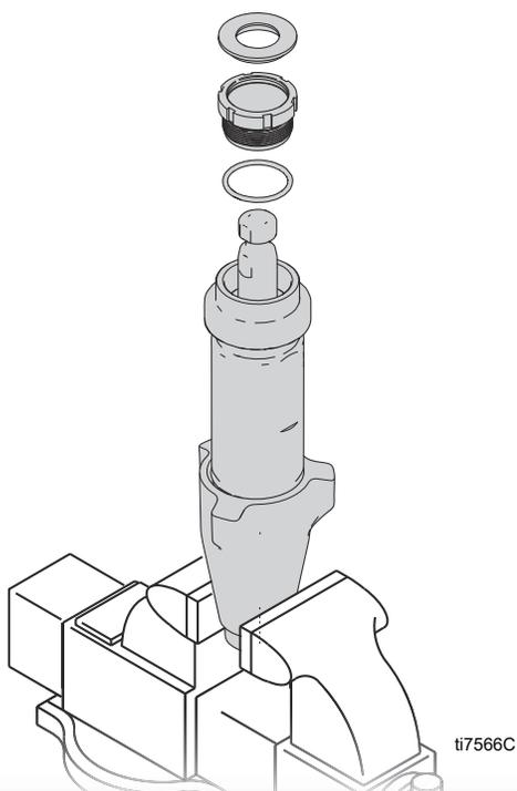
2. Unscrew intake valve from cylinder.
