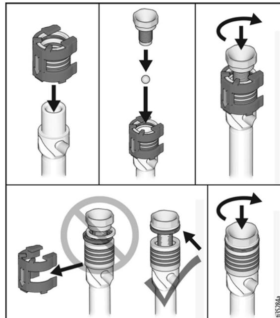
15. A) For all non-QuikPak Repair Kits. Soak all leather packings in SAE 30W oil for one hour minimum prior to assembly. Stack male gland (219) on piston rod. Alternately stack UHMWPE (208) and leather (218) packings (note orientation) on piston rod. Install female gland (217). Install piston wiper (216) and backup washer (229) (note orientation) on piston valve (210). The special sealing patch on
