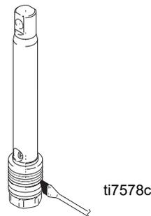
**NOTE:** Do not slide piston assembly into top of sleeve as this may damage piston packing.
