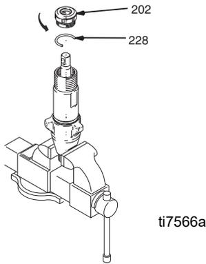
2. Unscrew intake valve from cylinder.
