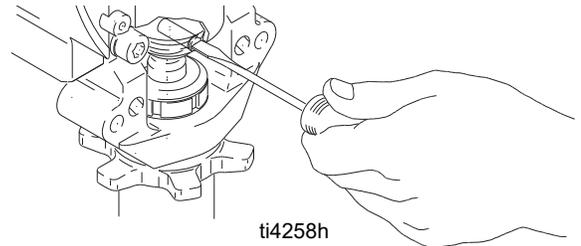
13. A) For all non-QuikPak Repair Kits. Soak all leather packings in SAE 30W oil for 1 hour minimum prior to assembly. Stack male gland (204). Alternately stack UHMWPE (203) and leather (223) packings (note orientation). Install female gland (224). Install seal (201) and packing nut (202) and o-ring (228).
