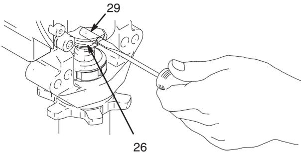
24. Reassemble intake valve with new o-rings (227), seat (212), and ball (214). Seat may be flipped over and used on other side. Clean seat thoroughly.
