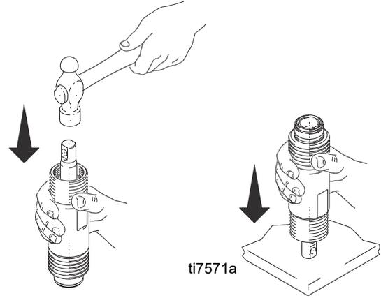
5. Remove piston rod from sleeve, or remove sleeve from cylinder. **Mark IV and Mark VII models:** Remove sleeve spacer (230) from sleeve.
