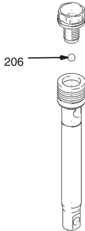
3. Tighten piston valve to piston rod as specified:
