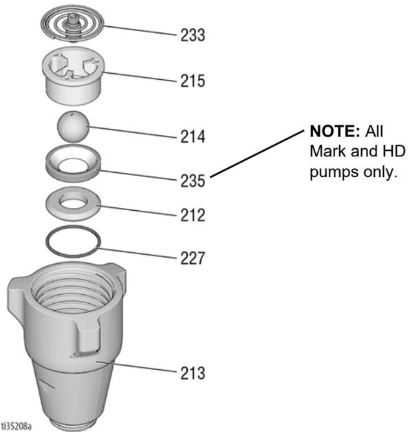
12. Install intake valve on cylinder. If a wrench is used torque as follows:
