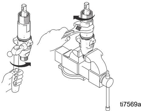
13. Torque packing nut (202) as follows:
