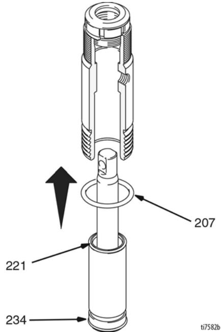
8. Grease top inch or two of piston rod that will go through the cylinder throat packings.
