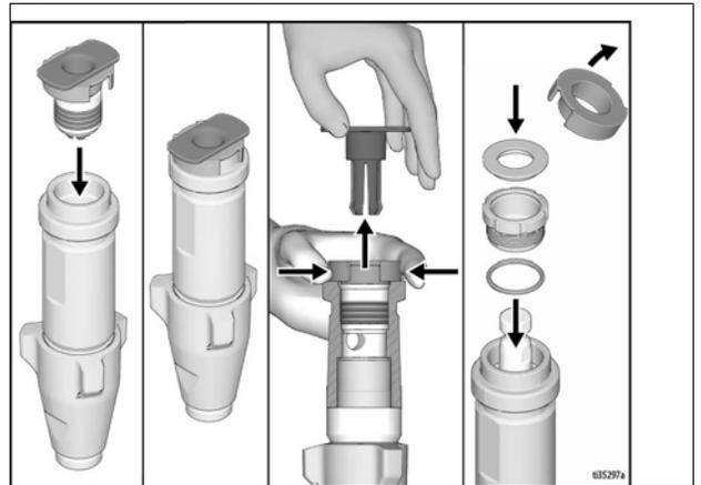
5. Install seal (201) into packing nut (202). Install o-ring (228) onto packing nut. Loosely install packing nut into cylinder.
