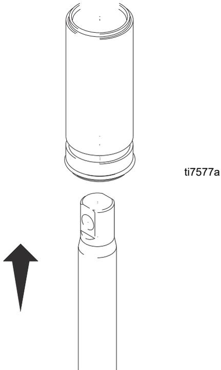
9. Grease o-rings (221 and 234) and place on sleeve. Slide sleeve/piston rod assembly into bottom of cylinder. Replace o-ring (207) if desired.
