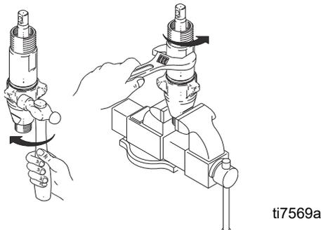
3. Disassemble intake valve. Clean and inspect o-ring (227).
