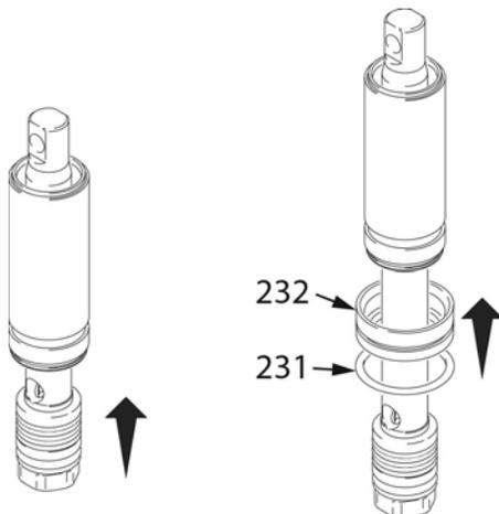
19. Grease top inch or two of piston rod that will go through the cylinder throat packings.
