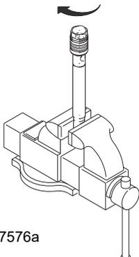
4. A) For all non-QuikPak Repair Kits. Soak all leather packings in SAE 30W oil for one hour minimum prior to assembly. Place male gland (204) in cylinder. Alternately stack UHMWPE (203) and leather packings (223) (note orientation). Place female gland (224) in top of cylinder seat packings.
