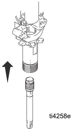
10. Insert piston rod into cylinder with pin hole up and piston valve down. Insert pin into piston rod and crank shaft.
