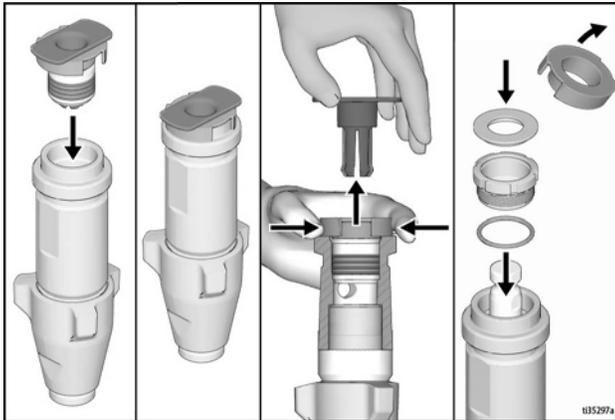
piston valve threads is good for four repackings. Use thread sealant on piston valve threads after four repackings.
