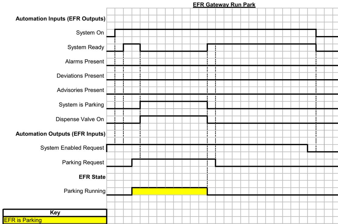
When the Parking Request bit is ON, the EFR will start parking as long as the System On bit is also ON. If the System On bit or the Parking Request bit is OFF, the EFR will stop parking.
