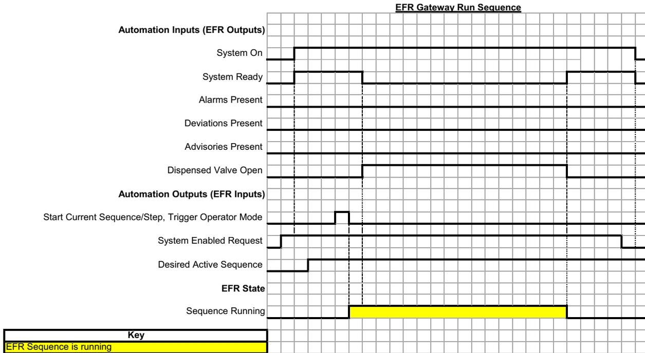
If the sequence is not in operator mode, a pulse on the Start Current Sequence/Step, Trigger Operator Mode bit will play the active sequence.
