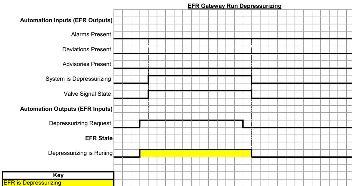
When the Depressurizing Request bit is ON, the EFR will start depressurizing. The EFR will only stop depressurizing if the Depressurizing Request bit is OFF.
