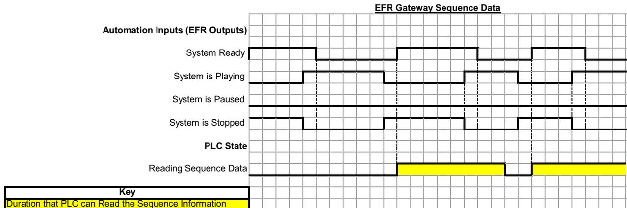
The Sequence Data must be read before the EFR finishes running another sequence. If the Sequence Data is not read before finishing the sequence, the data will be overwritten with new Sequence Data.
