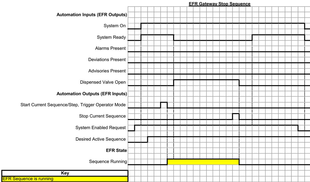
An ON pulse across the Stop Current Sequence bit will stop the active sequence.
