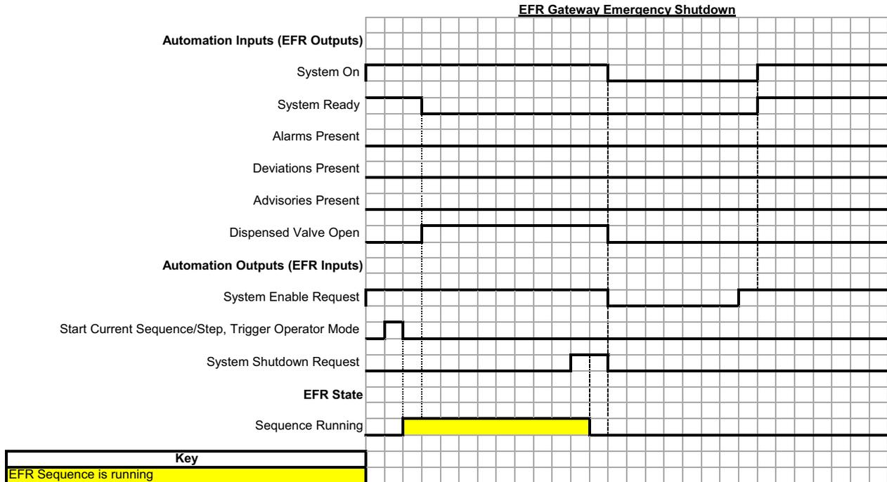
An ON pulse across the System Shutdown Request bit will stop the sequence and turn the System On bit OFF, making the system inactive.
