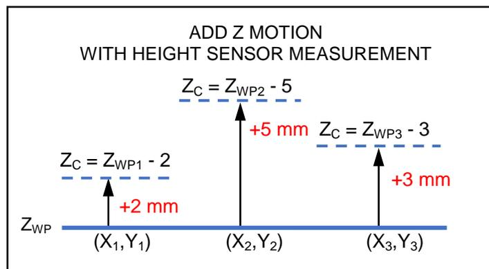
**Figure 15-1: Height Sensor Measurement Performed at  $(X_1, Y_1)$ ,  $(X_2, Y_2)$ , and  $(X_3, Y_3)$**
