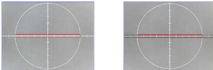
Figure 3-8: 500 Micron Horizontal Bar Measuring Tool (L); Measuring Tool Over a Fiducial (R)
