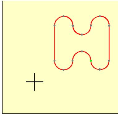
Figure 21-15: Missing Arc
