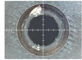
Figure 5-3: Prime Cup Center Enclosed by Grid
