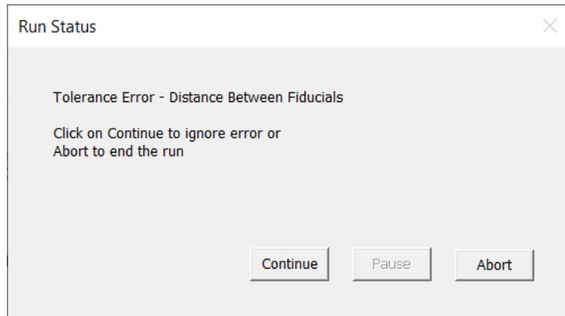
**Figure 16-8: Distance Between Fiducials Exceeds Tolerance**
