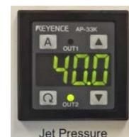
Figure 5-31: Set Jet Pressure to 40 psi.
