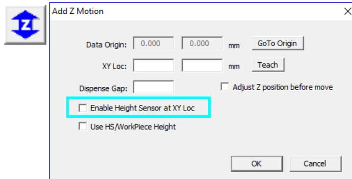
Figure 15-5: Height Sensor Option Not Used
