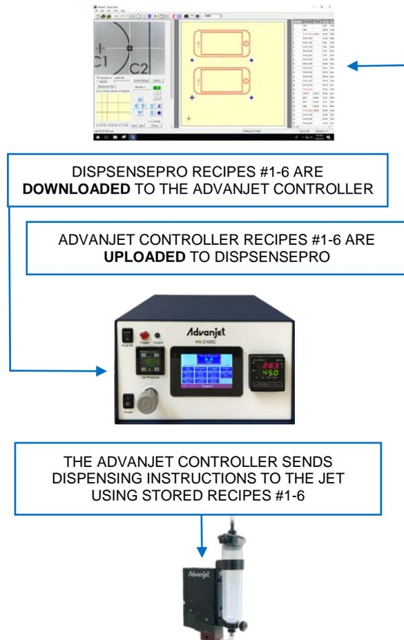
Figure 6-2: The Jet Dispenses the Recipes Stored in the Advanjet Controller
