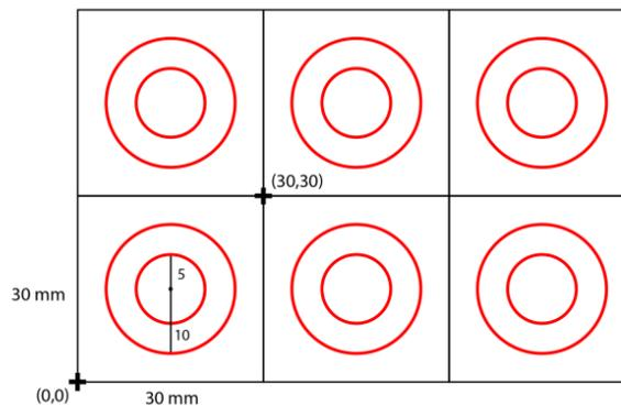
Figure 18-4: Two Rows and Three Columns of the Two-Circle Pattern
