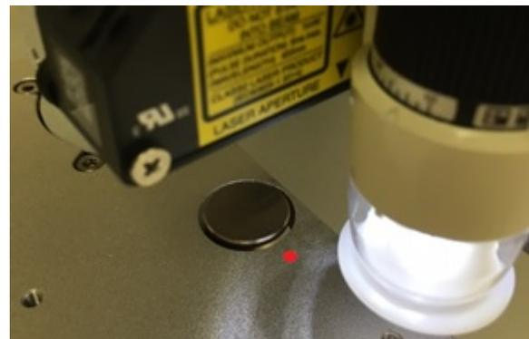
Figure 5-21: Laser Dot on Fiducial Marker
