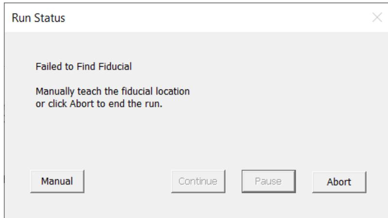
Figure 16-6: Failed to Find Fiducial
