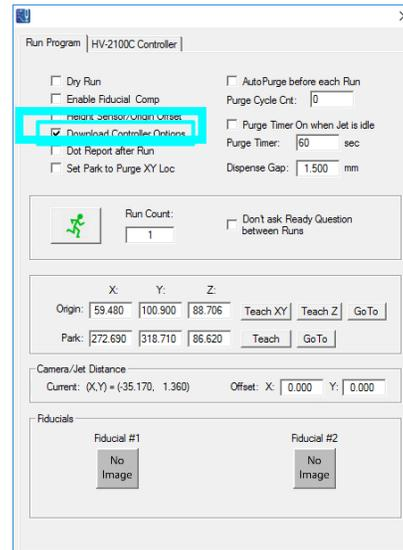
Figure 6-4: Select Download Controller Options in the Run Window
