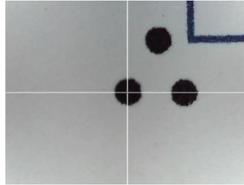
**Figure 16-9: Poor Fiducial Selection;
