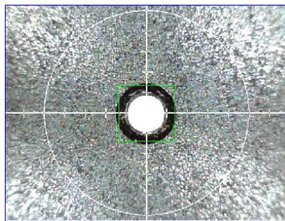
Figure 5-11: Green Box Tightly Encloses Fiducial Marker
