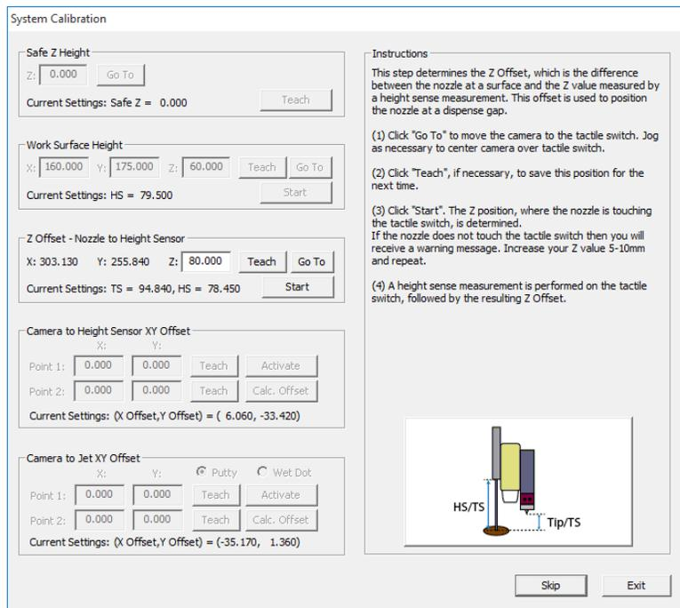
Figure 5-16: Nozzle Tip to Tactile Switch
