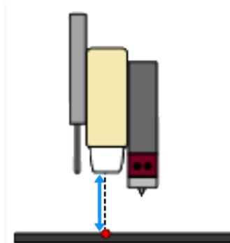
Figure 7-1: Z Focus Height is the Z-Axis Position When the Camera Image Is In Perfect Focus
