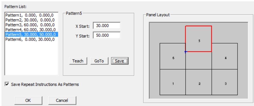
Figure 18-2: Start Point of Pattern5 Changed from (30,30) to (30,50)
