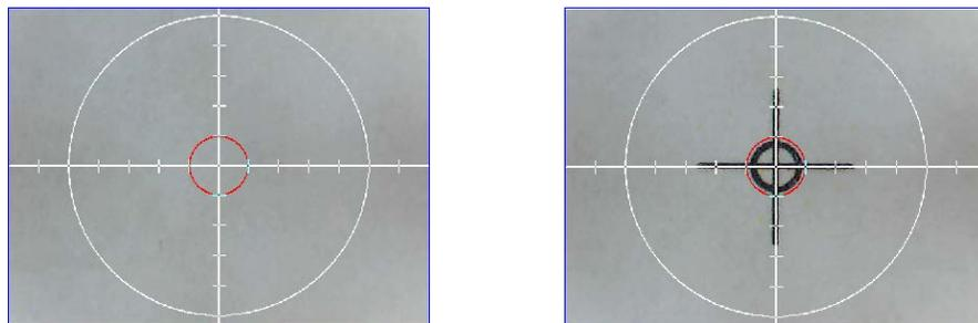
Figure 3-7: 1200 Micron Circle Measuring Tool (L); Measuring Tool Over a Fiducial (R)
