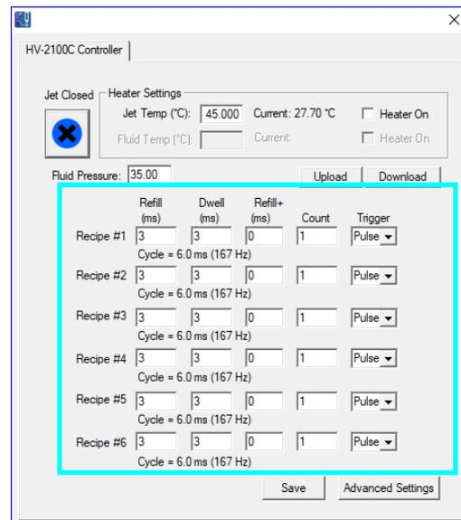
Figure 20-6: Timing Recipe Parameters
