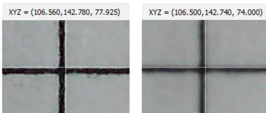
Figure 7-2: Robot's Z In Z Focus Position (L); Robot's Z Not In Z Focus Position (R)
