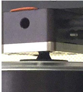
Figure 5-28: Jet Nozzle Tip Positioned on Prime Cup
